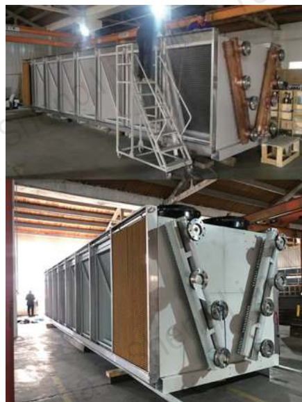
Country: USA Application: Bitcoin immersion cooling system Cooling capacity: 1270kW Cooling medium: BC-888 Supply power: 415V/3P/60Hz Fan brand: Ziehl-Abegg
