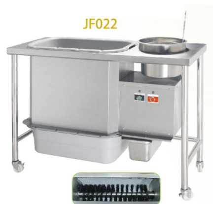
Rotating brush, automatic coating powder
