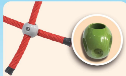
Item Code: SDN-ALU-002 Name: Solid Cross Connector(Small) For 16mm combination rope Made of casting aluminium (0.059kgs) To connect 2pcs ropes in a cross
