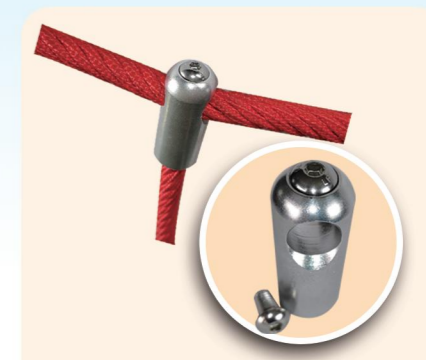
Item Code: SDN-ALU-015 Name: Aluminium T Connector Material: Aluminium Fix two sections of 16mm six strand- -steel wire rope Screw hole: 16mm
