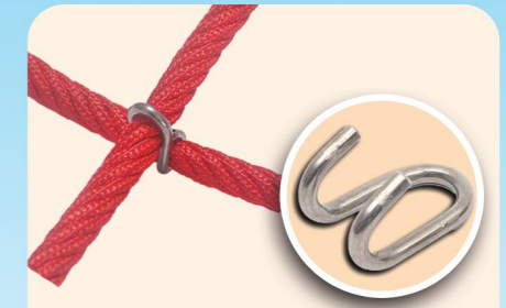
Item Code: SDN-STA-003 Name:Stainless steel double hook Made of dia.5.0 mm 304 steel (0.031kgs) To fasten 2pcs Dia.16mm rope in a -crossed way
