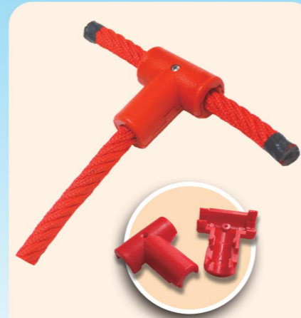
Item Code: SDN-NYL-001 Name: Nylon T-Connector(split type) For 16mm combination ropes Made of injection moulded PA (0.060kgs) It consisting of two parts are unre- -movable after assebly
