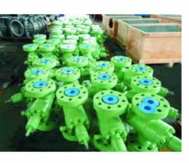
All gate and seat materials and coatings are functionally tested in a 10,000 psi valve, with blow-downs at full differential pressure. The test valve is opened with a pneumatic actuator, which opens the valve much faster than hydraulic or manual operation and provides the most rigorous test condition.
