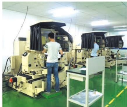
PG光曲磨 PG optical curve grinding
